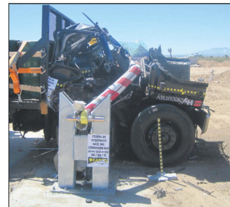
The StrongArm M30 halted the vehicle from 30 mph in less than 1 meter, earning it the highest M30 rating possible: P1, the company reports.
