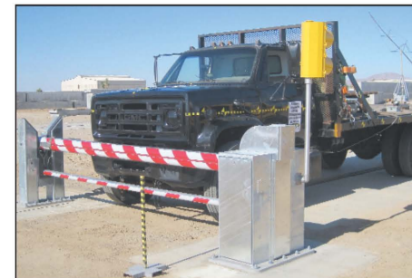
The GMC 7000 vehicle weighing 15,000 pounds is staged prior to the actual crash test. (HySecurity photos)
